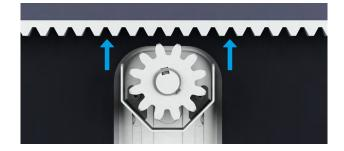
2. The pointer plate on the gear unit (2) pushes the upper limit indicator (3) upwards. The lower limit indicator (4) is pushed manually under the pointer plate.
