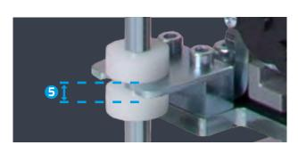
**4.** The distance between the two limit indicators (**5**) can be easily measured.
